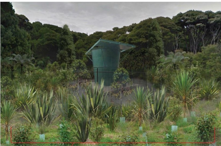
Above: An underground mine on Conservation land could be accessed from outside the area and could require only a vent shaft showing on the surface in the bush.
